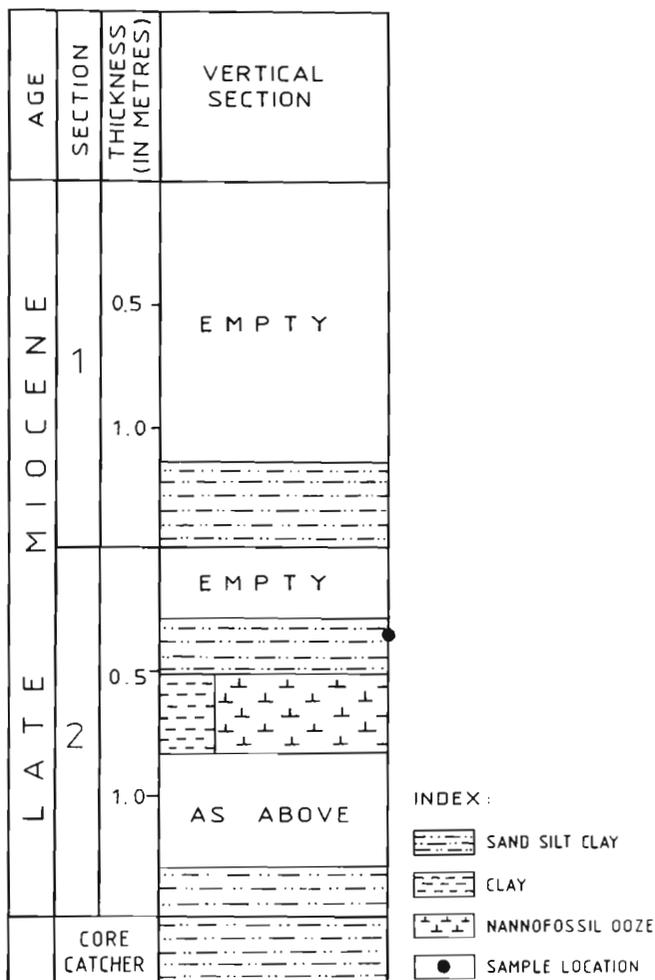
Text-figure 2—Core 16 of DSDP Site 218 showing location of sample.
