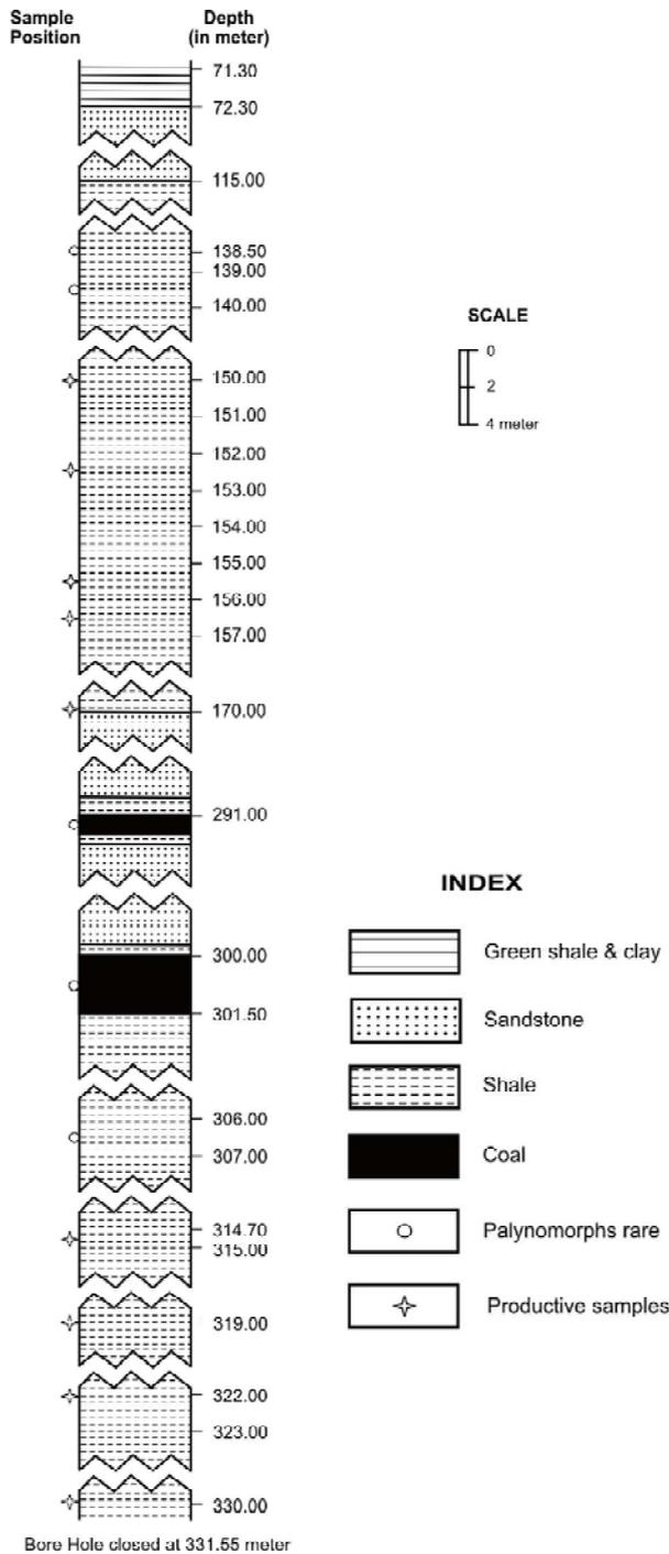
Fig. 3—Lithological details of the samples collected from Bore hole No. MR-157, Makardhokada area, Nagpur District, Maharashtra (Courtesy, DGM, Nagpur).
