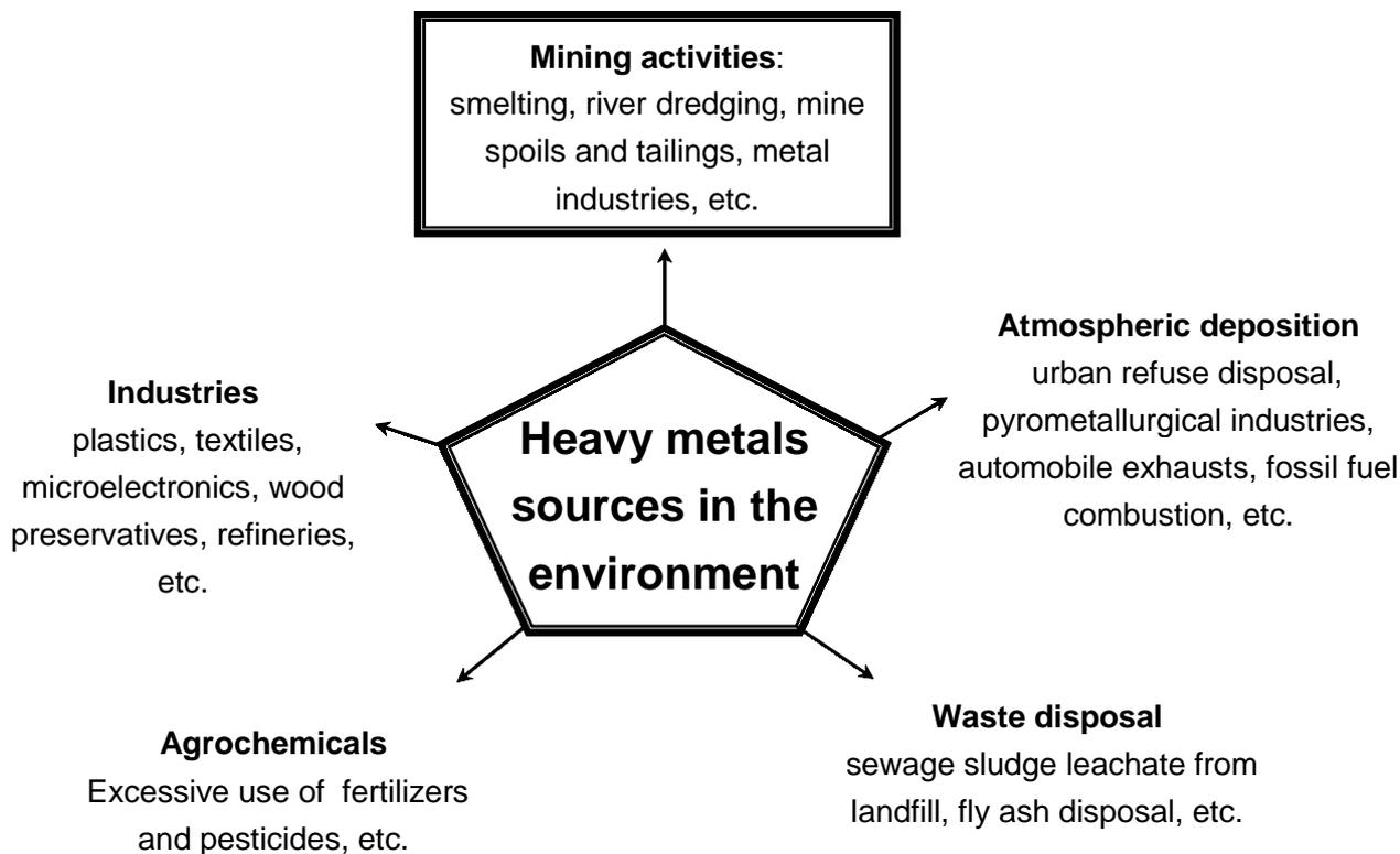
Fig. 1—Environmental exposure of heavy metals due to mining and related technogenic activities.
