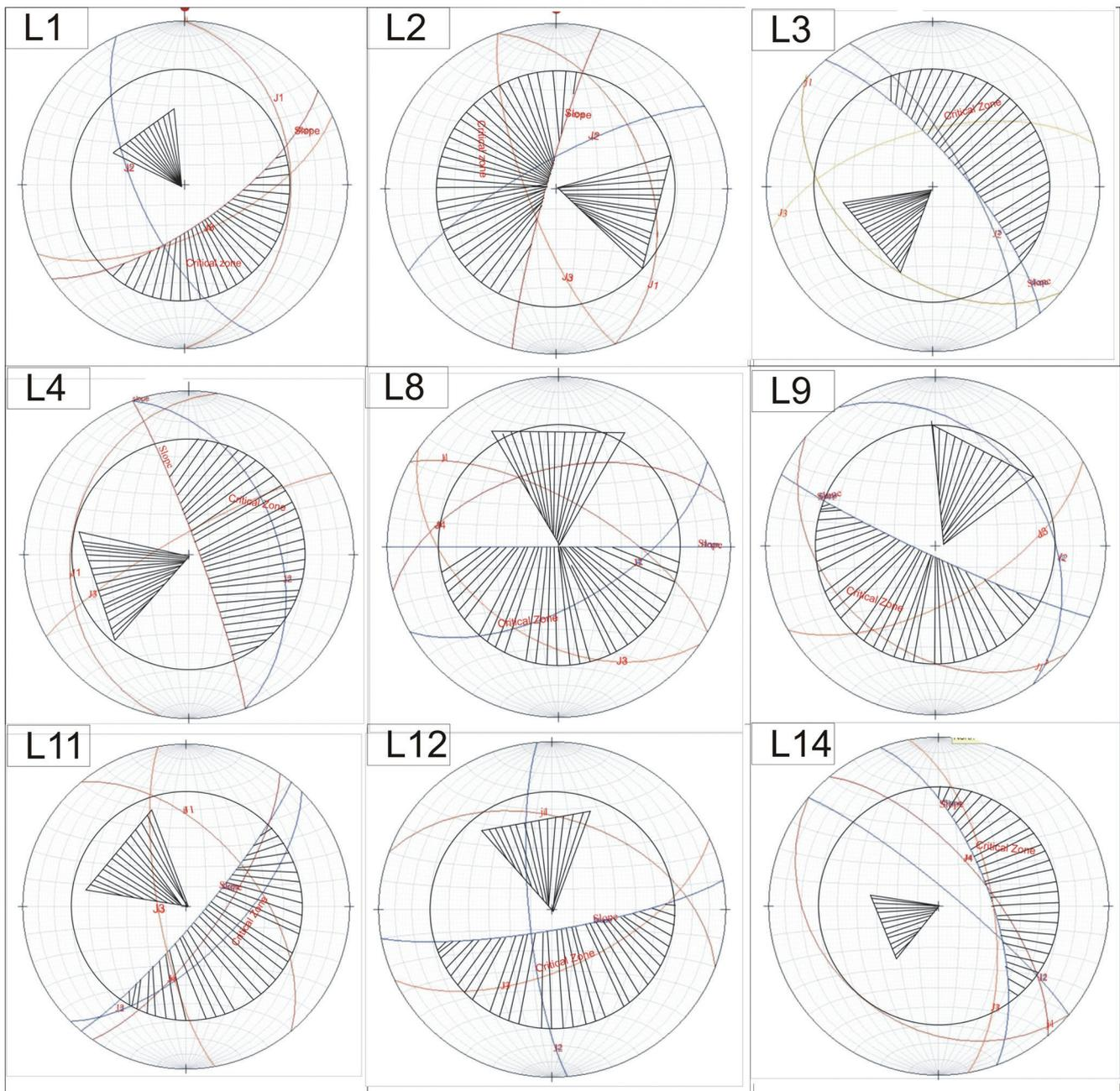
Fig. 3—Graphical presentation of geometrical relationship between slope face and discontinuity data recorded at different locations in the study area.
